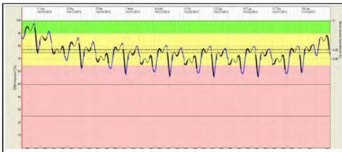
Figure 23. Predicted Effectiveness of a 5-on/10-off, 3-section watch rotation. (Hollins and Leszczynski, 2014, p. 28)
