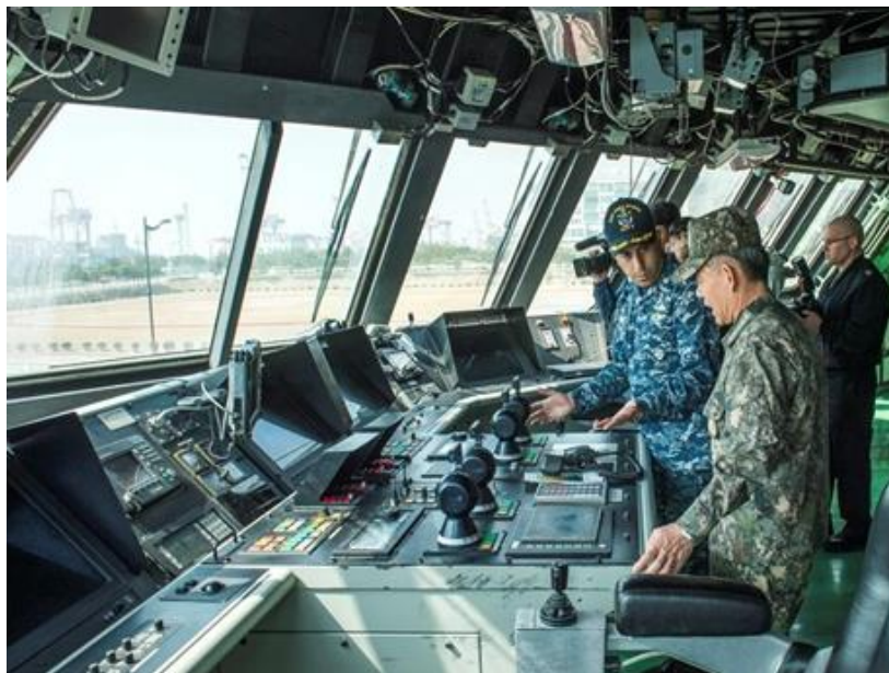
Figure 3. Photograph of LCS Bridge showing Human-Automation Interface equipment (IBS) (Source: U. S. Navy)
