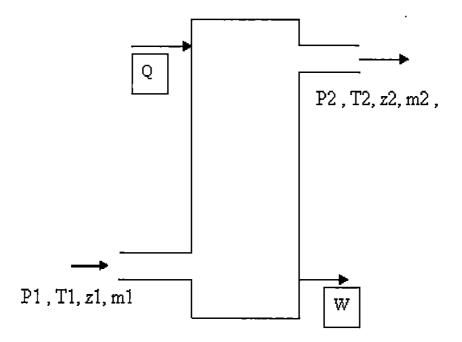
Fig. 4.1 Schematic representing an open system
