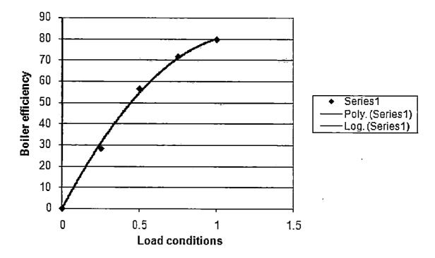
Graph 4.2 Boiler efficiency Vs. Load conditions for Coal fired boiler
