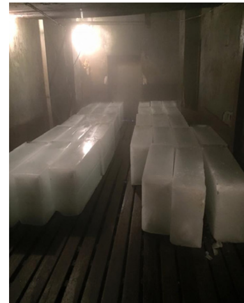
The ice blocks are then stored in a cold room to a temperature of 17.6°F (-8°C).
