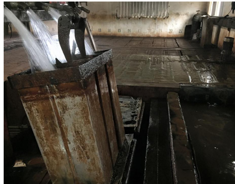
The empty ice tanks are refilled with water and put back to freeze at the temperature of 23°F (-5°C).
