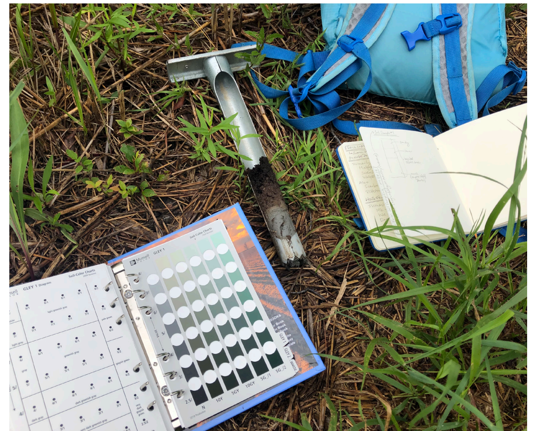
Fig. 12: Assessing soil colors with a Munsell soil chart Haile Farm Preserve, Warren, RI
