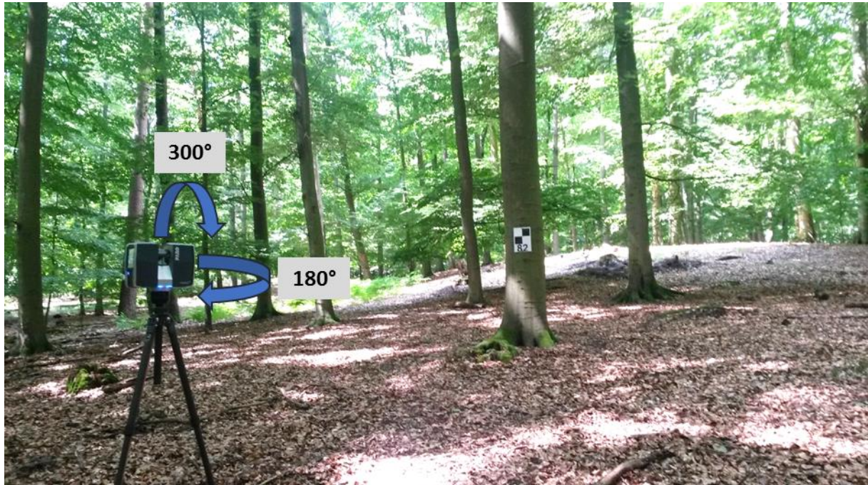
Figure 1.2: The principle of terrestrial laser scanning: the scanner is mounted on a tripod and turns 180 degrees in horizontal direction and 300 in vertical direction, providing a field of view of 360 \times 300 degrees.
