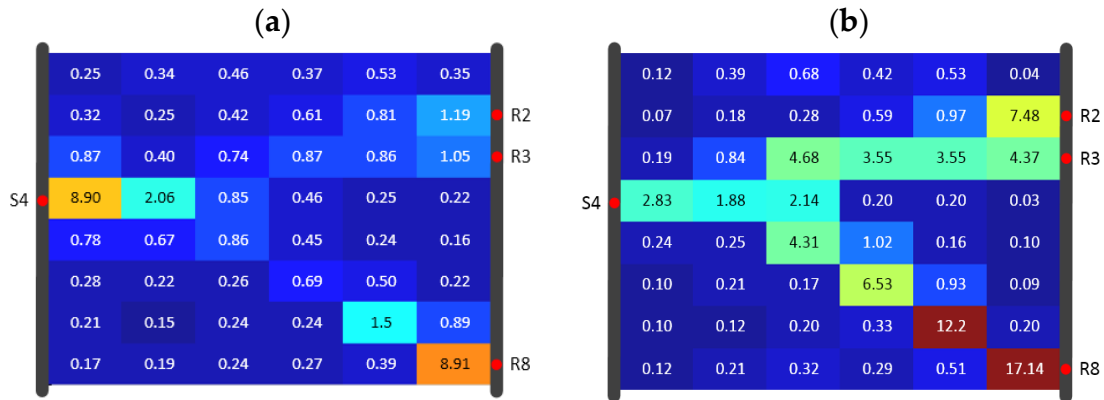
Figure 3.15. Algorithm result comparison for the model under 8 \times 6 resolution of the (a) SIRT result and (b) SIRT-Cimmino result, shown in diffusivity [ \text{m}^2\text{s}^{-1} ].
