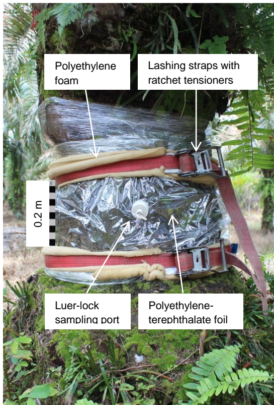
Figure A2 A stem chamber attached to an oil palm stem.
