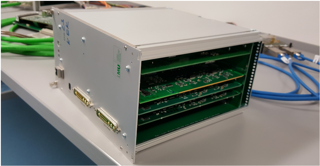
Figure 4.19.: Photograph of an LMU power supply unit.
