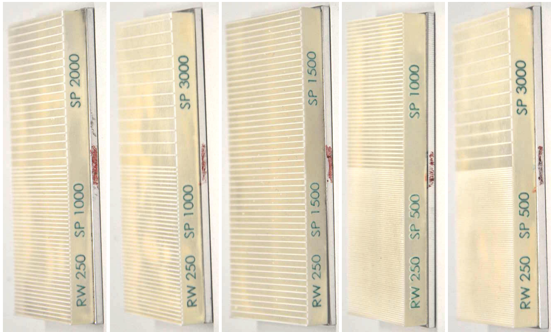
Figure 2.17: Photos of the stimulation plates used for the passive stimulation task. The different grated stimuli used in the passive stimulation task. Ridge width for all stimuli was 250\mu\text{m} . Each plate had a different spacial pacing on the two sides. Spacial pacing (left-right) for the five stimuli was 1000\text{-}2000\mu\text{m} , 1000\text{-}3000\mu\text{m} , 1500\text{-}1500\mu\text{m} , 500\text{-}1000\mu\text{m} and 500\text{-}3000\mu\text{m}
