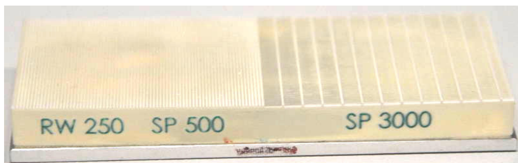
Figure 2.16: Close-up of one stimulation plate used for the passive stimulation task. The different grated stimuli used in the passive stimulation task. Ridge width for all stimuli was 250\mu\text{m} . Each plate had a different spacial pacing on the two sides. Spacial pacing of the shown stimulus was 500\text{-}3000\mu\text{m}
