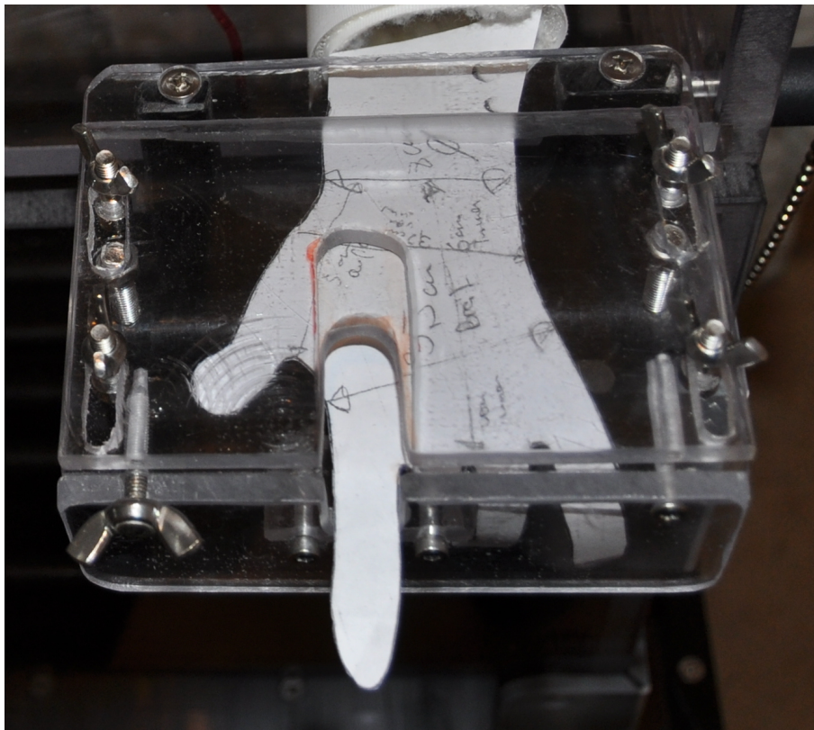
Figure 2.15: Photo of the hand holder. A photograph of the hand holder. The animal places his hand around a bar (below the paper hand) and has to extend one finger through the hole at the front of the hand holder. Plates around the hand restrict movements to avoid that the animal accidentally comes into contact with moving platform parts.
