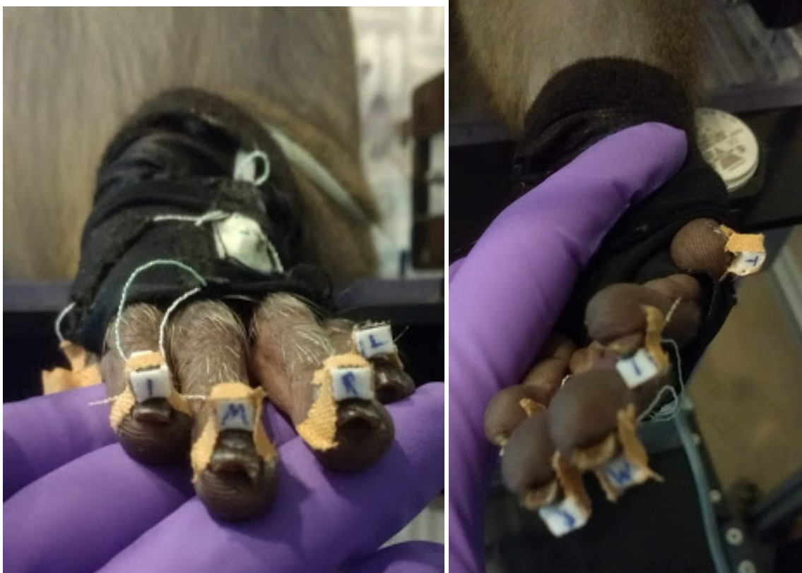
Figure 2.10: Photos of the kinematic data glove, worn by monkey Ralph. Kinematic data glove (Schaffelhofer and Scherberger 2012). Pictures of monkey Ralph wearing the data glove, while the sensors (white and marked with letters) are glued to his fingertips using Leucotape. The Leucotape secures the white sensors from the top but leaves the finger tips free. Purple: The experimenters hand.
