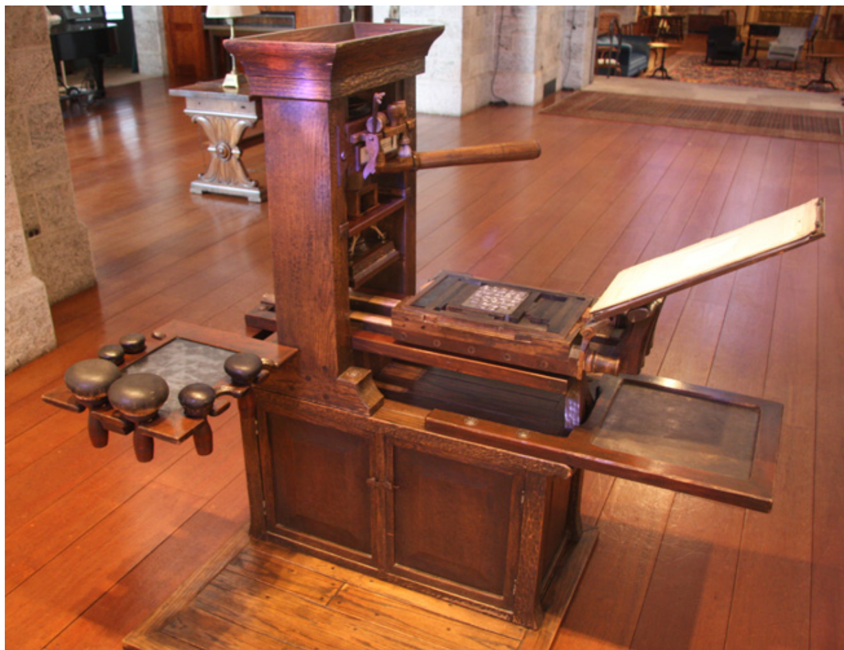
Figure 1: Glencairn's "Fenix Press," a replica Gutenberg-era printing press. Source: Glencairn Museum/
