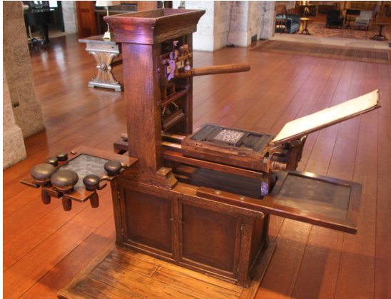
Figure 1: Glencairn's "Fenix Press," a replica Gutenberg-era printing press.
