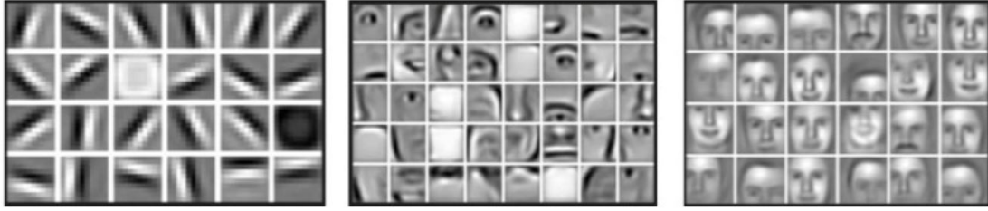
Figure 4. Sample of the feature maps generated by the CNN. At the first few layers, basic shapes are detected, and the deeper layers, higher level features are learnt
