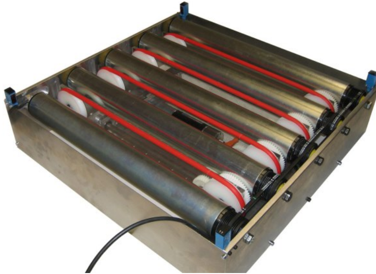
Figure 3: FlexConveyor (an individual module) (Uludağ, 2012). A FlexConveyor is able to receive an item from any side, and it can also move the item to any side. The rollers of a FlexConveyor move an item in one pair of opposite directions, and the belts move the item in the other pair of directions.
