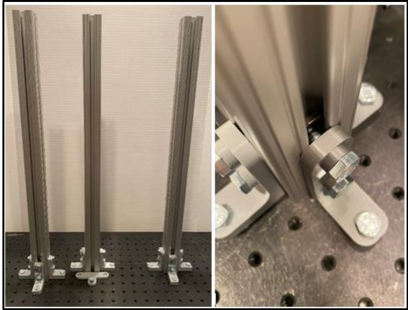
Figure 45. Assembly of major mount to optical bread board.
