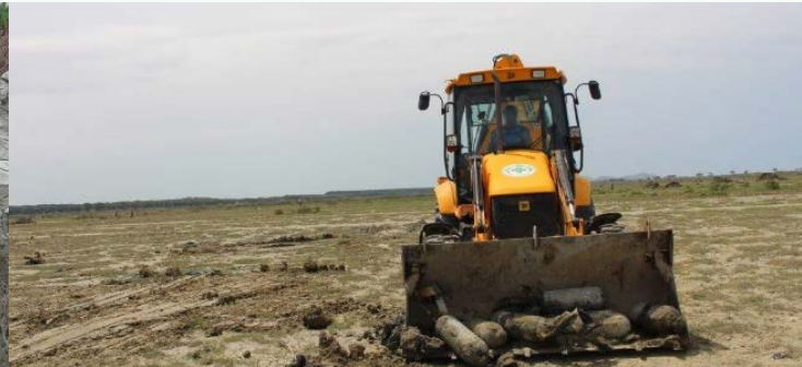
Anti-tank mine found in TD-HS-b site (depth of 15 cm). JCB assisting in removing located aerial bombs
