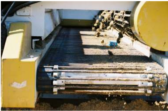
Figure A-17: Mine on Cross Conveyor
