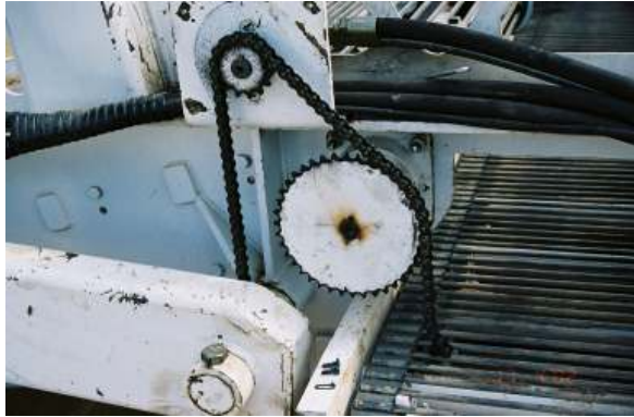
Figure A-22: Broken Drive Chain
