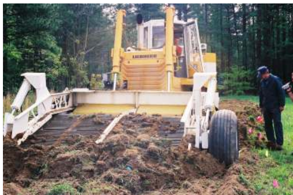
Figure A-14: HLS Sifting Light Clay and Sod
