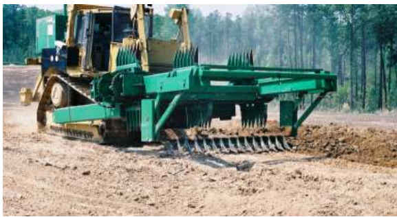
Figure A-3: Floating Mine Blade (out of ground)
