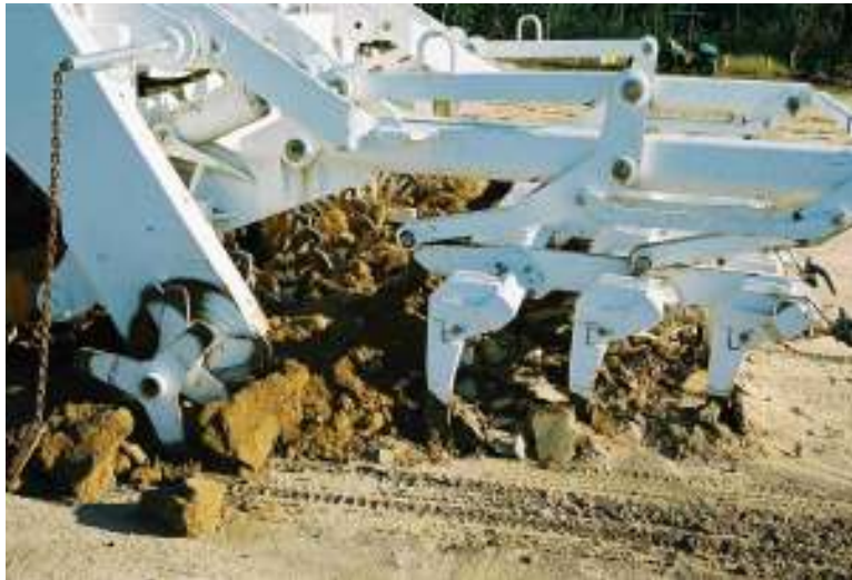
Figure 4: Mine Clearing Cultivator
