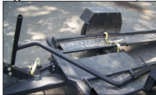
Figure 32: Trailer with Removable Handle (Handle is Lying on Trailer, Not Connected)
