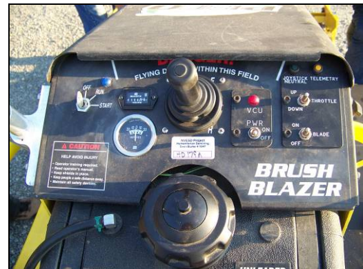
Figure 7: Instrument Panel After Modifications
