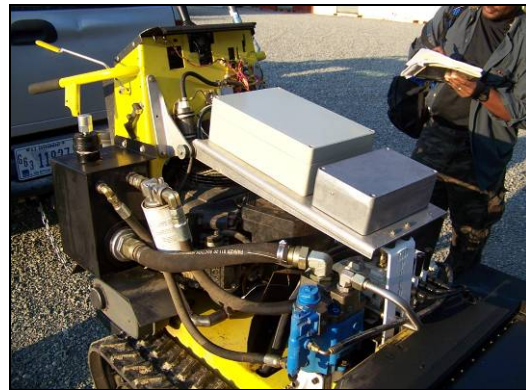
Figure 5: Peco Cutter Engine After Modifications (Top Cover Removed in Photo)
