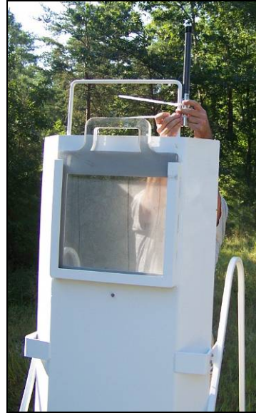
Figure 25: Mounting Remote Antenna to Operator Shield
