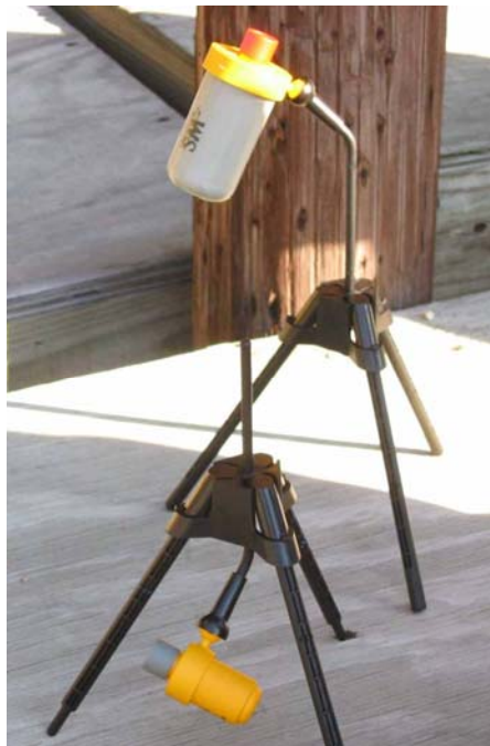
Figure 25: SM-EOD System Setup (33 above, 20 below)
