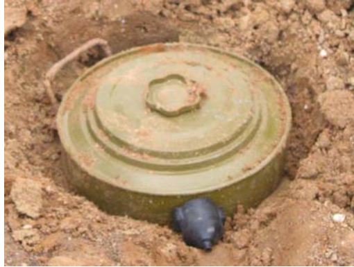
Figure 24: PESCO HD 22 g Perforator against a TM-46 Antitank Mine Target
