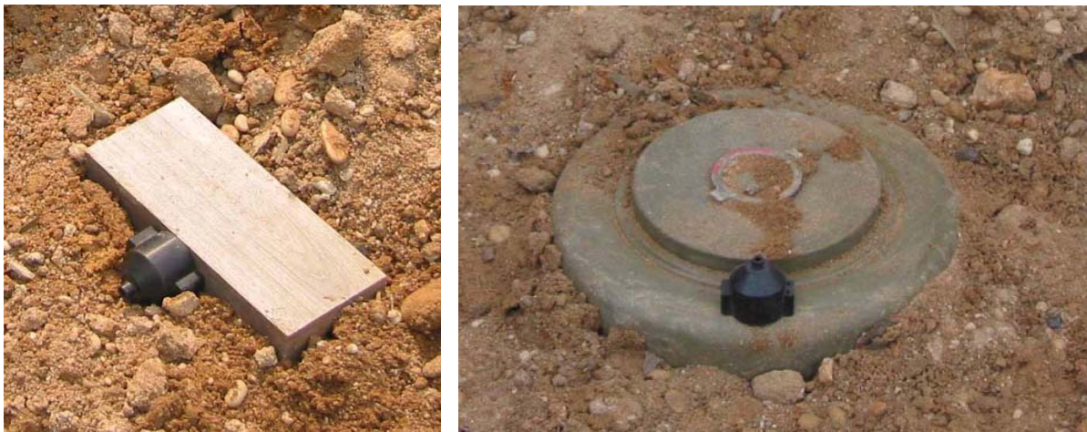
Figure 23: PESCO HD 11 g Perforator against PMD-6 Antipersonnel and Round Antitank Mine Targets
