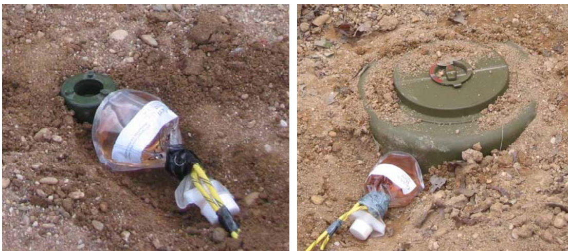
Figure 19: Liquid Explosive Pouch 1/2-pound Charges against T-AB-1 Antipersonnel and Round Antitank Mine Targets
