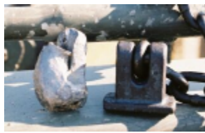
Picture 31 – A worn flail head (left, lost during run) and a new flail head (right)
