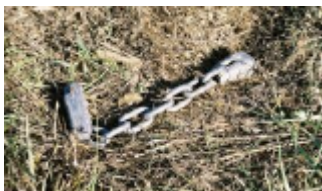
Picture 30 – Flail weight lost during run
