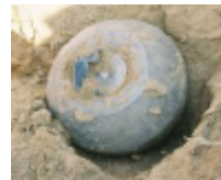
Picture 25 – Load cell with multiple dents
