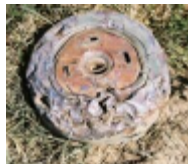
Picture 24 – AT mine with multiple dents
