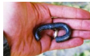
Picture 32 – Broken interlink
