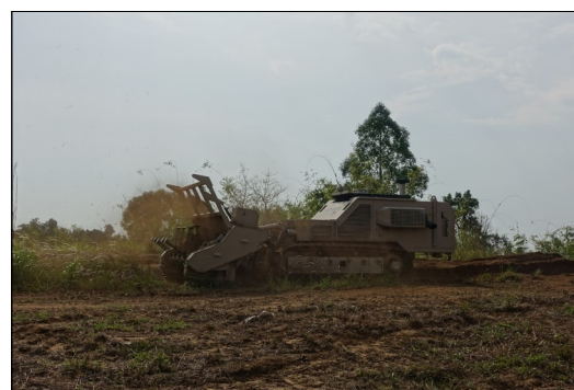
MEDIUM MW WITHOUT THE OPERATOR STATION OPERATING IN THAILAND
