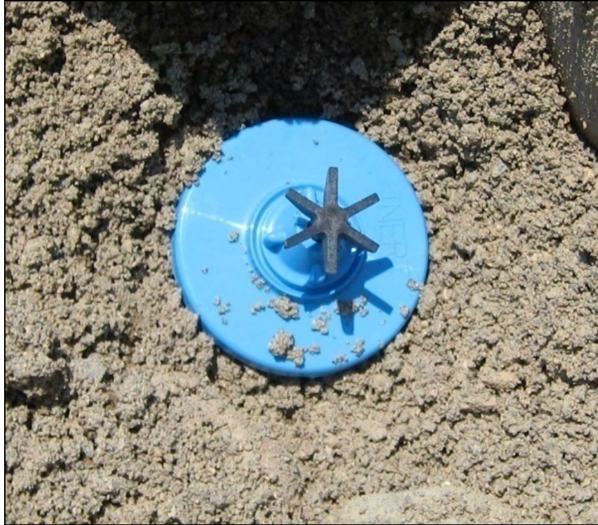
Figure 11: MRM Simulant, PMA-2 Antipersonnel Mine
