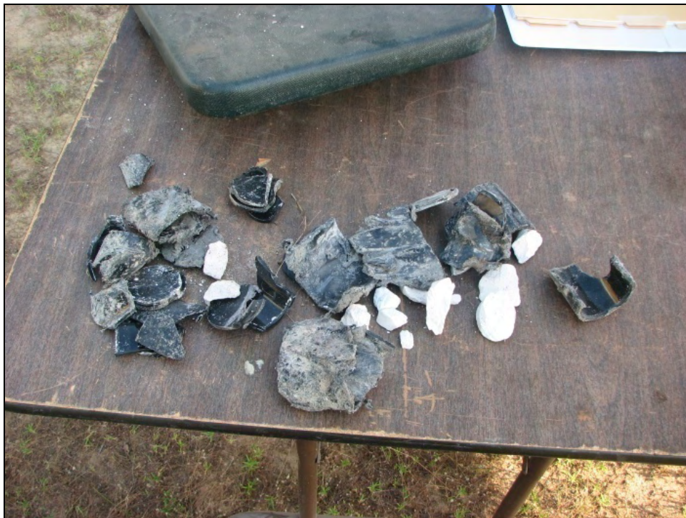
Figure 22: PVC Mine Simulants, 10 mm Setting
