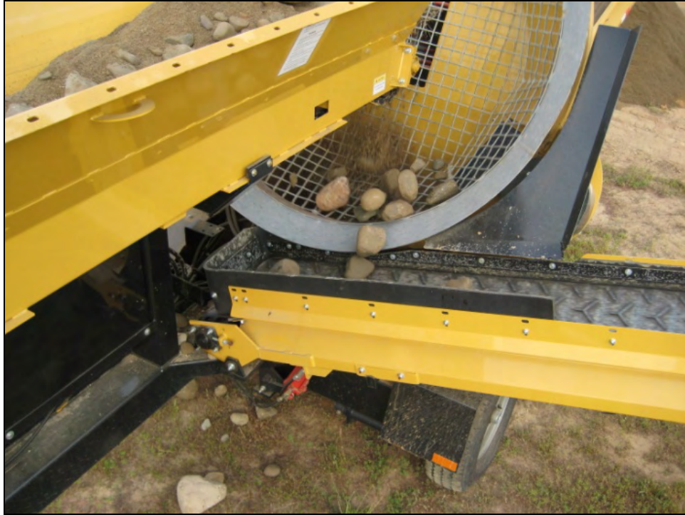
Figure 17: Material Exiting Screen onto Conveyor Belt
