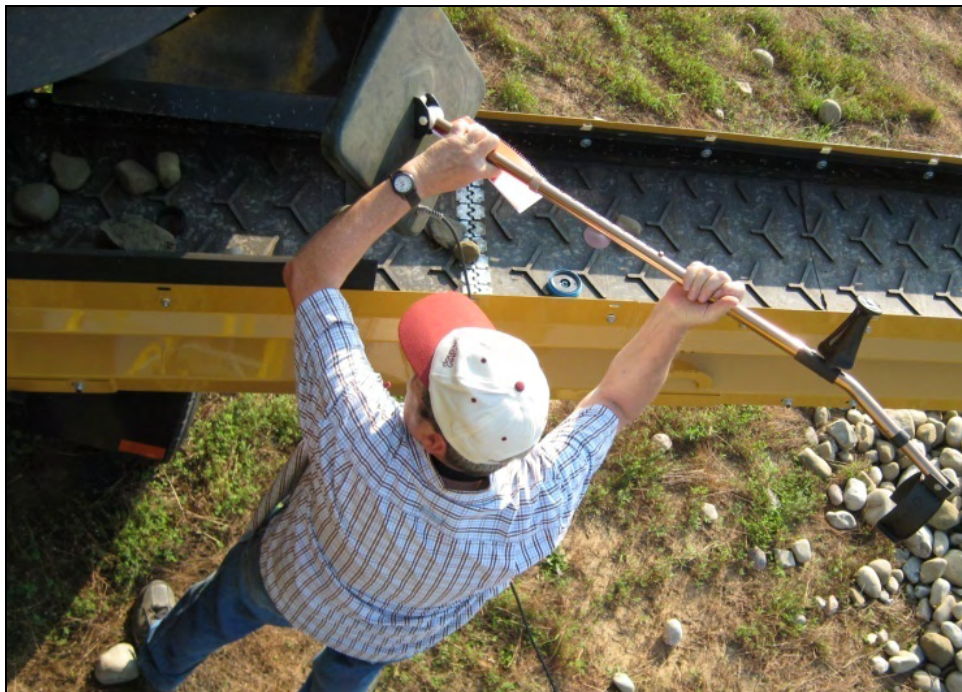
Figure 18: Scanning MRMs on Conveyor Belt
