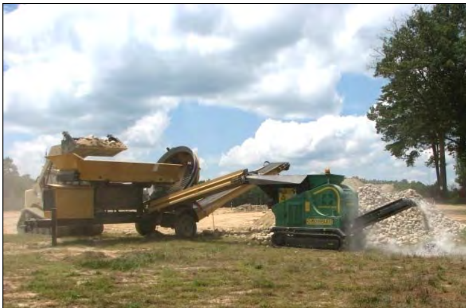
Figure 29: Sifter, Crusher Joint Operations
