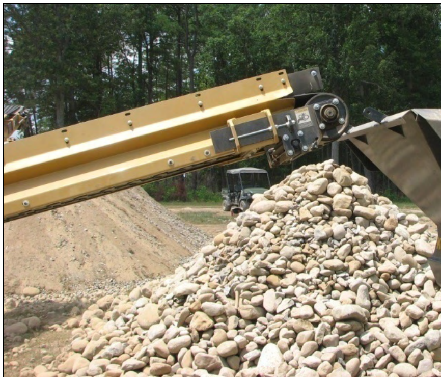
Figure 15: Sifted Material Exiting Conveyor
