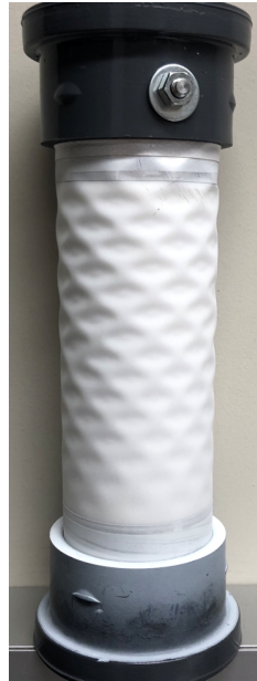
(b) Experimental apparatus with 50.8 \mu\text{m} shell.
