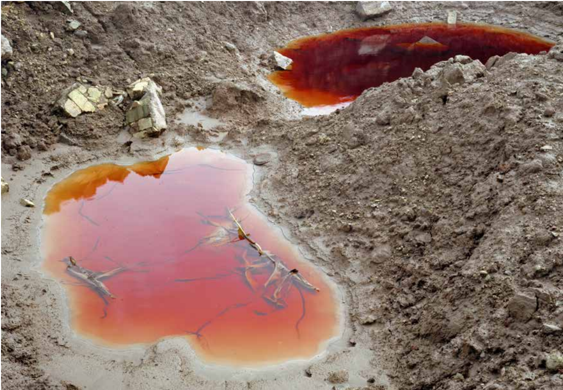
Puddles of so-called 'red water' photographed at an Iraqi army ammunition storage depot, Shykh Na Tm, Kumayt, Maysan Governorate, South Eastern Iraq, 2004. Red water is a waste product produced during the manufacture of the commonly used explosive TNT. Red water is hazardous because of the toxicity of its various constituents, for example some (e.g. dinitro-toluene) are probable human carcinogens and also have been known to have impacts on the blood, kidney, liver, and nervous system of exposed individuals. Photo: Jonathan Olley
