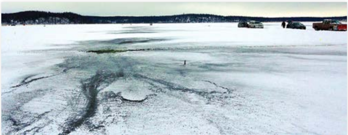
A detonation plume from a high explosive ordnance residue test in Alaska. Snow is the perfect medium for measuring the environmental deposition of energetics. Researchers at the Cold Regions Research and Engineering Laboratory (CRREL) used various techniques to simulate low-order detonations with both traditional and insensitive high explosives fillings.
