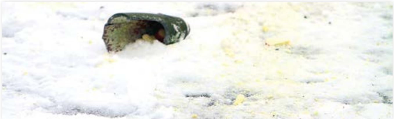
IMX-104 fill spread after a low-order technique. Second order and low order techniques are prone to leave more residue. Researchers at the CRREL in Alaska have used various techniques to simulate low-order detonations with insensitive high explosives fillings.
