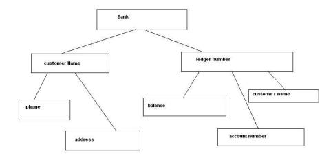
Figure 2.5: Parent child relationships in the hierarchical database model [5]
