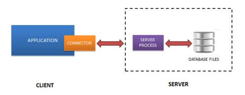
Figure 7.7: Client server architecture [2]
