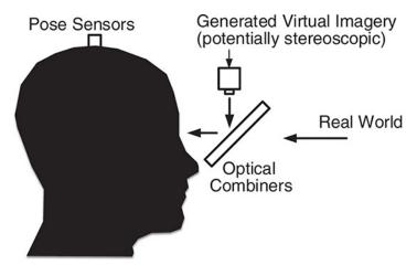
**Figure 2.4:** How real-world imagery is transmitted to the eye using an optical see-through display (Illustration by Schmalstieg and Höllerer. In *Augmented Reality: Principles and Practice.*)
