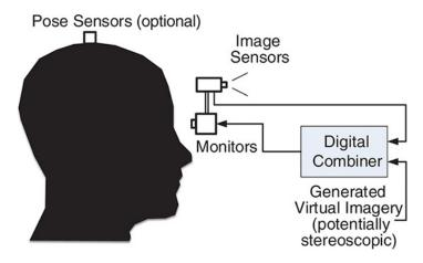
**Figure 2.5:** How real-world imagery is transmitted to the eye using a video see-through display (Illustration by Schmalstieg and Höllerer. In *Augmented Reality: Principles and Practice.*)
