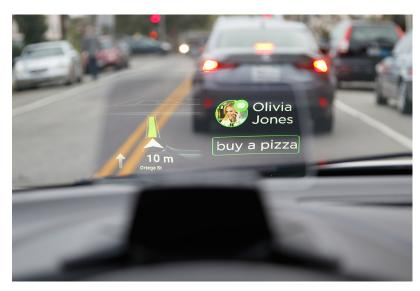
**Figure 2.7:** A map projected by the head-up display HUDWAY Drive on a car's windshield (Photograph by HUDWAY.<sup>18</sup>)
