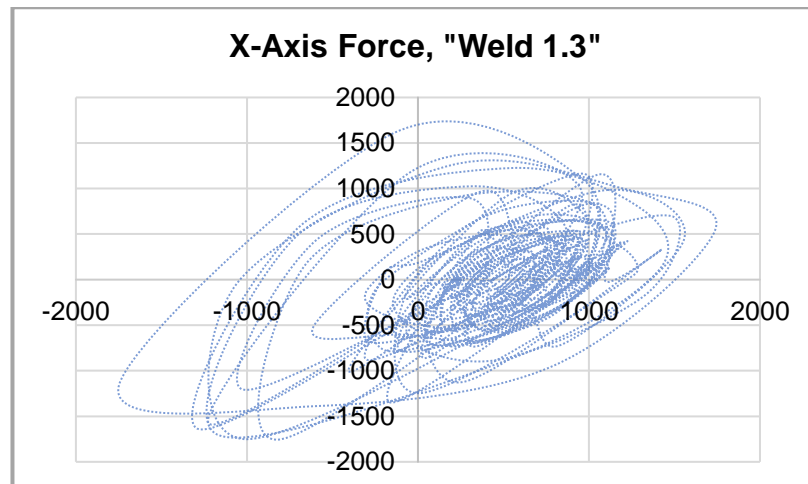
Figure 5.18: "Weld 1.3" Phase Space plot of Spindle Longitudinal Force
