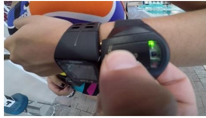
Figure 24: Photo illustration of the green light activation of the GeneActiv tri-axial accelerometer, during the video and accelerometer synchronization method within the present study.
