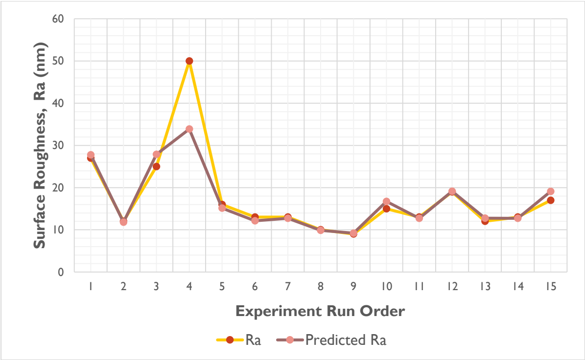
Figure 4.13: Comparison of measured and predicted surface roughness of the RS model 1
