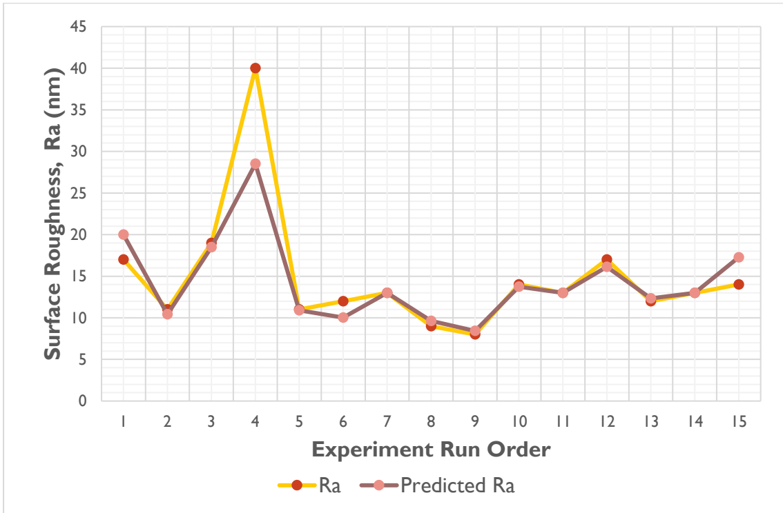
Figure 4.14: Comparison of measured and predicted surface roughness of the RS model 2
