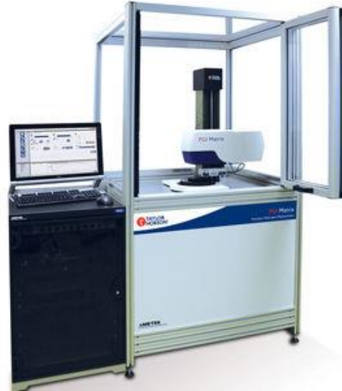
Figure 3.12: Taylor Hobson PGI Dimension XL Surface Profilometer
