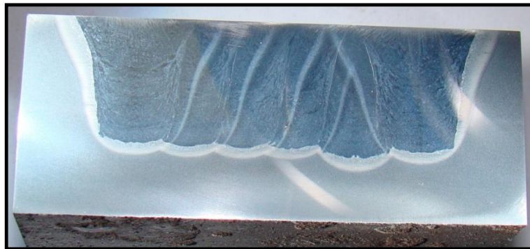
Figure 1-1. Linked Blind FTSW in 30mmSteel (Taken at NMMU)
