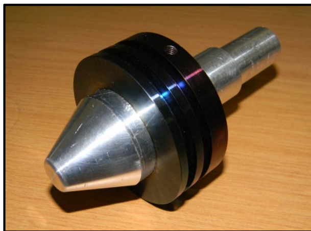
Figure 5-1. Steel (EN-8) Heat Sink
