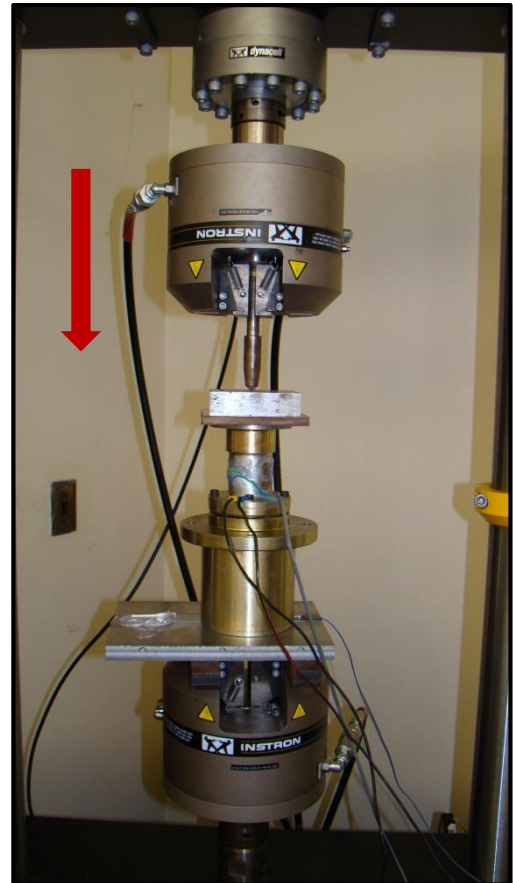
Figure 3-6. Axial Force Component Calibration Setup
