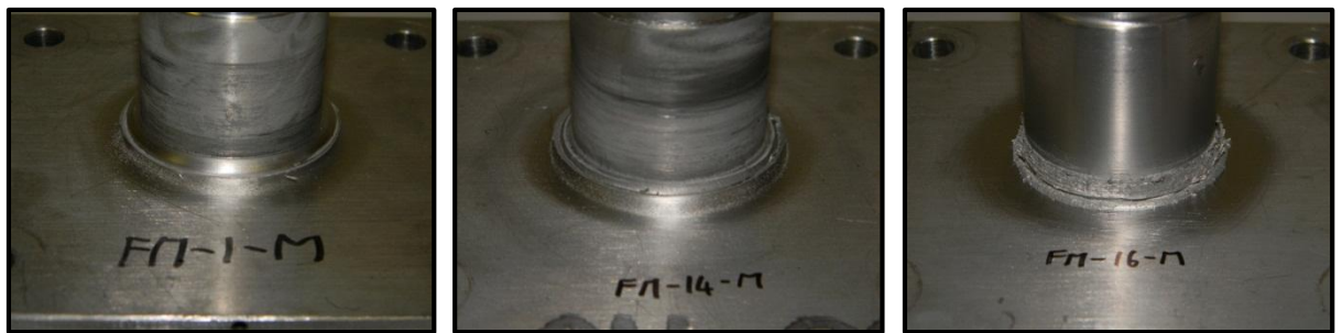
Figure 5-31. Flash Formation of Welds FM-1 to FM-16
