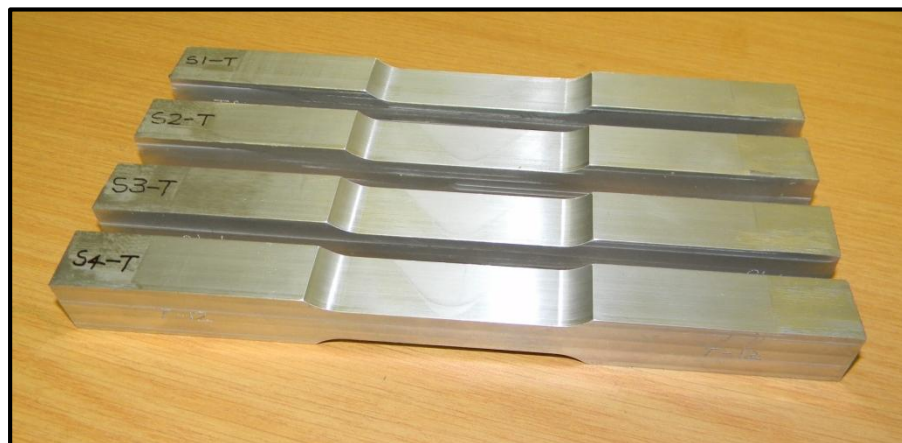
Figure 5-8. Tensile Samples of Welds S.1 to S.4
