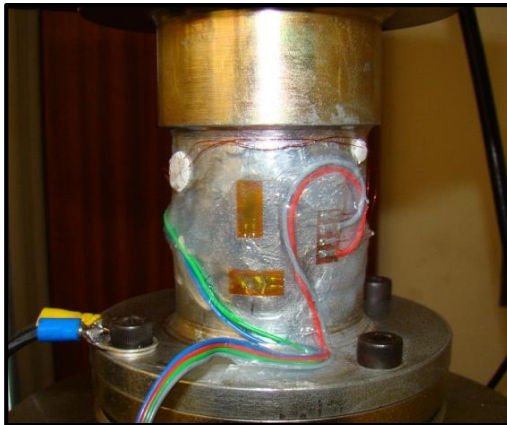
Figure 3-5. Strain Gauges Fitted to Axial Force Component
