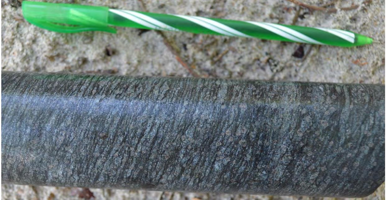
Figure 22: Medium-grained grey foliated garnet biotite schist showing garnet porphyroblasts within a biotite and calcite rich matrix. The foliation is defined by fine-grained dark grey biotite; light grey bands are calcite and quartz.
