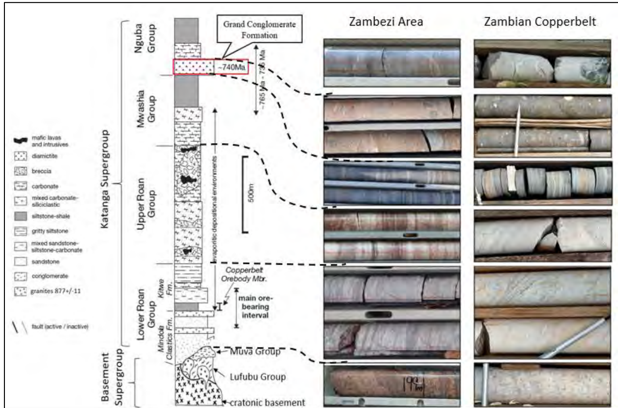
Figure 71: Stratigraphic succession of the Katanga Supergroup and the basement with correlating photographs of the Zambezi area and the eastern and central Zambian Copperbelt (modified after Selley et al., 2005).
