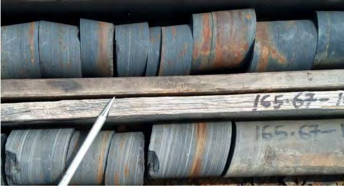
Figure 7: Finely laminated grey shale interlayered with light grey carbonate and brown oxidized pyrite.
