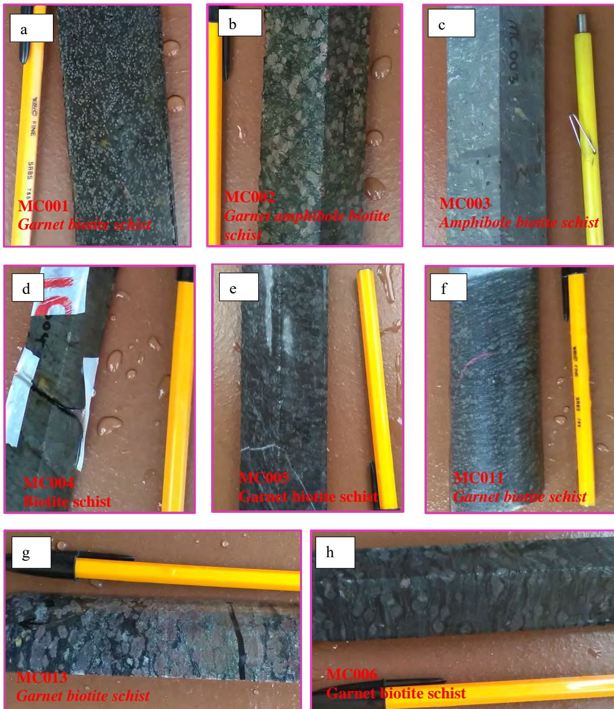
Figure 31: Core samples from different holes of various biotite schists and garnet biotite schists selected for petrographic analysis. All samples belong to the Grand Conglomerate Formation. (a) Weakly foliated grey garnet biotite schist composed of biotite and calcite matrix with randomly distributed pink ~1 mm garnet porphyroblasts. (b) Porphyroblastic garnet amphibole biotite schist. Matrix is fine-grained grey biotite and calcite with pink garnet and grey amphibole porphyroblasts. (c) Massive grey amphibole biotite schist, amphiboles are randomly oriented within a calcitic
