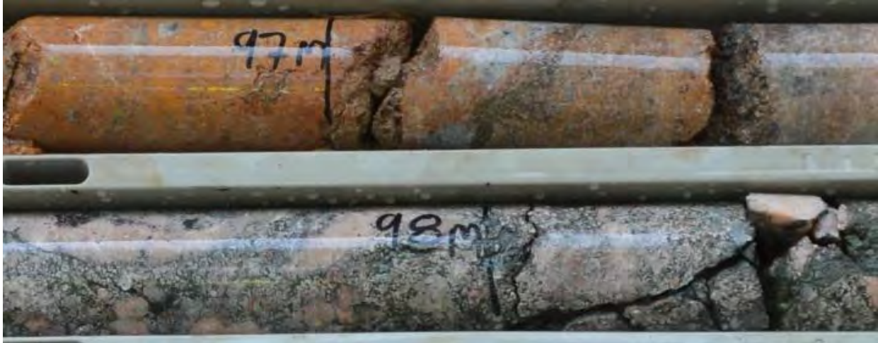
Figure 20: Carbonate breccia consists of two different compositional breccia. The brown breccia with carbonate clasts cemented by carbonate and iron oxide matrix while the grey breccia has carbonate clasts cemented by biotite rich matrix.
