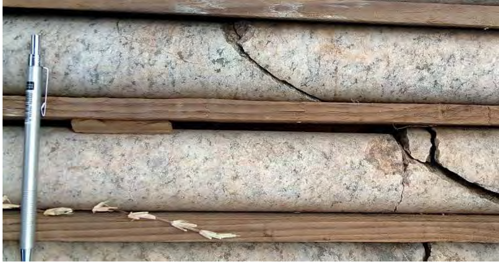
Figure 4: Pink coarse-grained meta-granite composed of feldspar, quartz, biotite and muscovite. It is weakly sheared with semi-continuous biotite bands.
