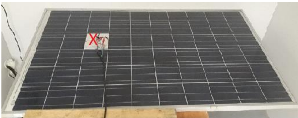
Figure 4. 10: Module under test inside the environmental chamber, X is an aluminium plate measuring 157mm x 157mm x 3mm, placed on a cell surface and biased to positive terminal of the power supply.
