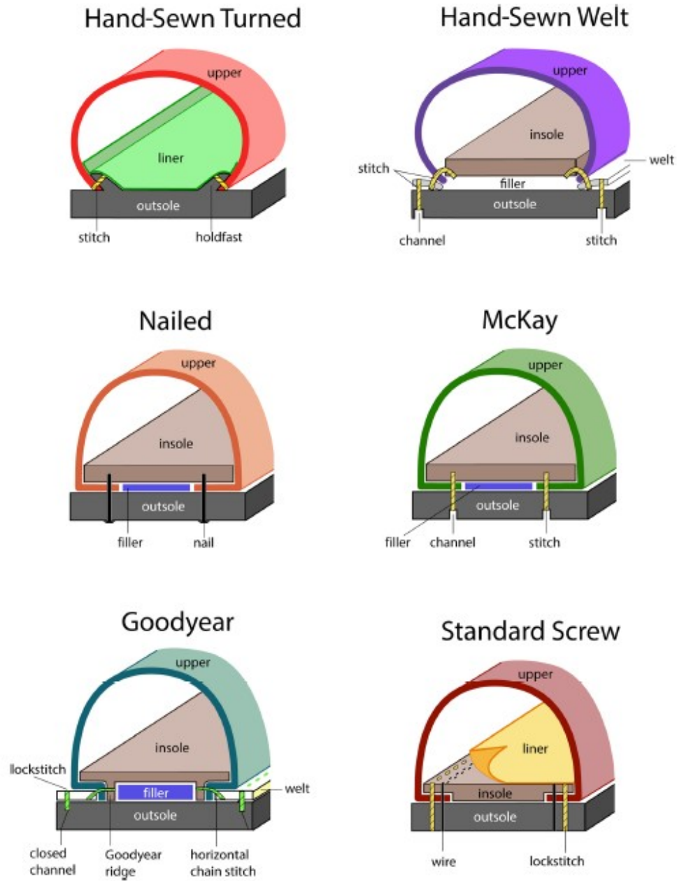
Figure 4.10: Illustration of footwear construction Morphology. After Dappert-Coonrod and Mihich (2018:650)
