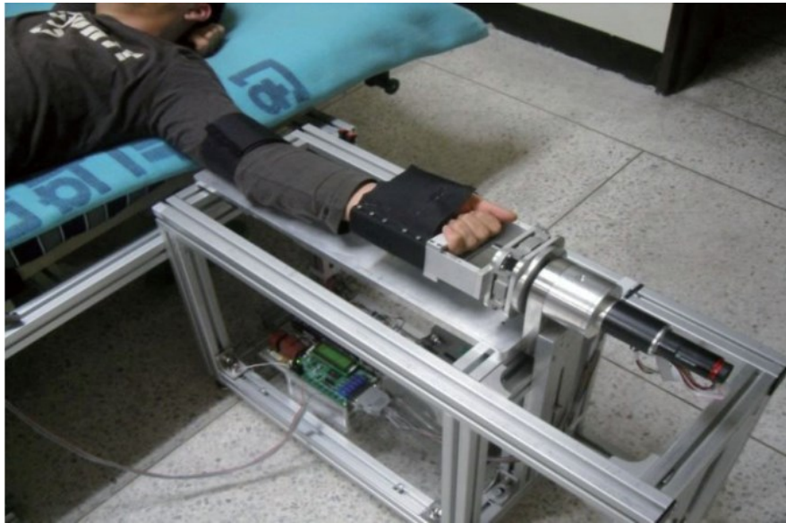
Figure 2.1 Experimental setup of Wrist Rotation Rehabilitation Robot [13]
