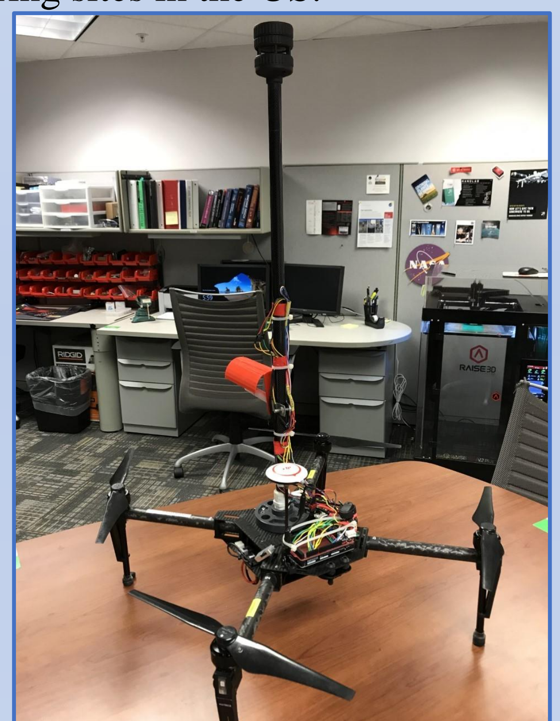
Figure 3: M-100 UAV used for flying the OPC-N3 sensor.
