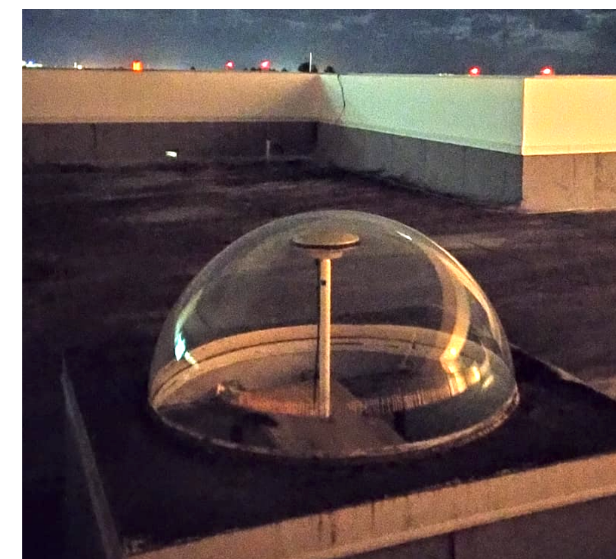
Figure 2: One of SPRL's GPS-703-GGG antennas on top of the COAS Building at ERAU
