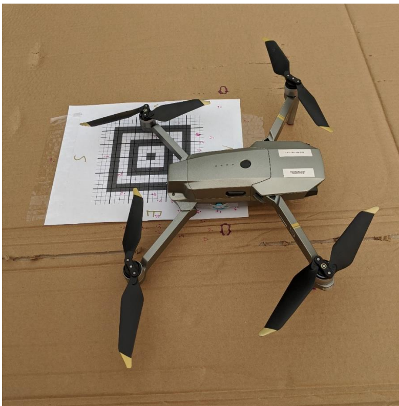
Figure 8. An example of a marked landing point after the drone motors stopped.
