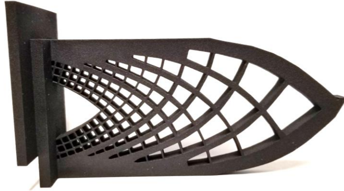
Figure 5.5 Optimized cantilever beam test specimen as printed by MJF.
