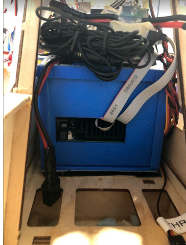
Figure 3.3 PCM 3356 and Analog board enclosed in 3D Printed Box
