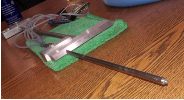
Figure 4.2 ADP is assembled with sting, rod and mounting block with pneumatic tubes
