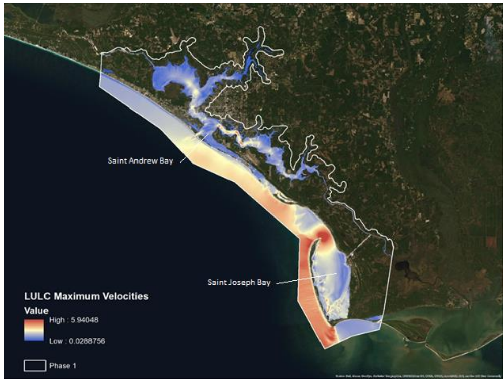
Figure 4.5 a. Maximum water velocities (m/s) produced in the LULC scenario.
