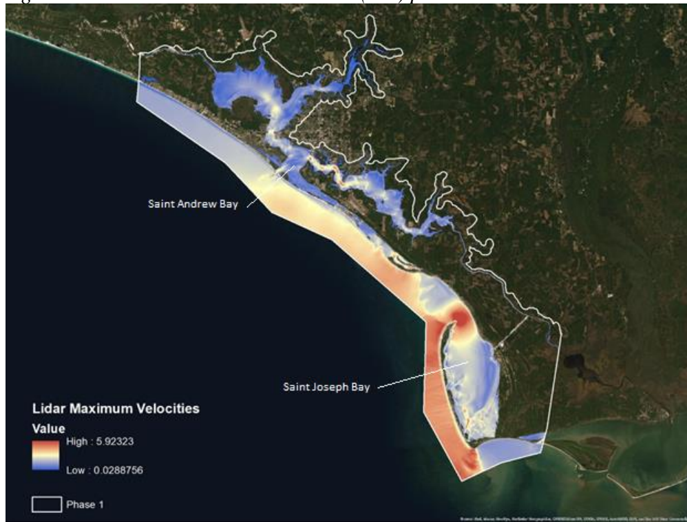
Figure 4.5 a. Maximum water velocities (m/s) produced in the LULC scenario.
