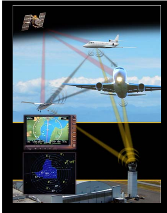
Figure 1.2 ADS-B schematic diagram (“Automatic dependent surveillance – broadcast”, n.d.).
