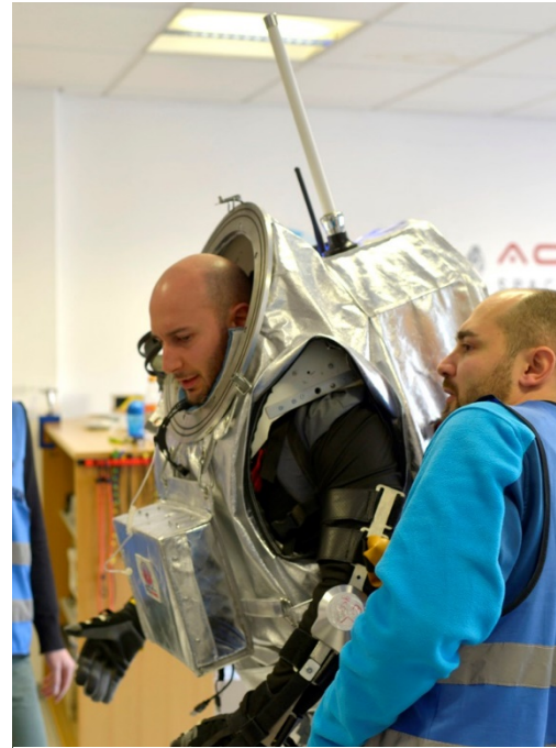
Figure 10: Internal view of the Aouda.X suit at AMADEE-18 showing the shoulder joint of the exoskeleton [ÖWF, 2016].
