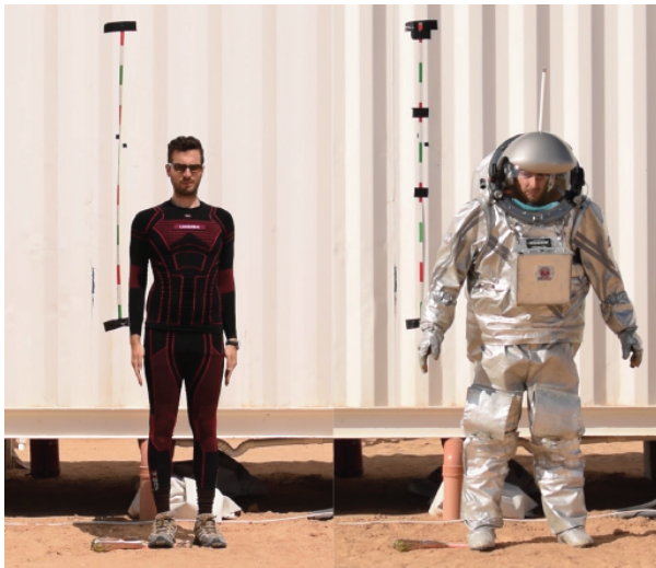
Figure 11: Unsuited and suited visual difference between neutral position for shoulder adduction B17 test for the AMADEE-18 Aouda.X suit.
