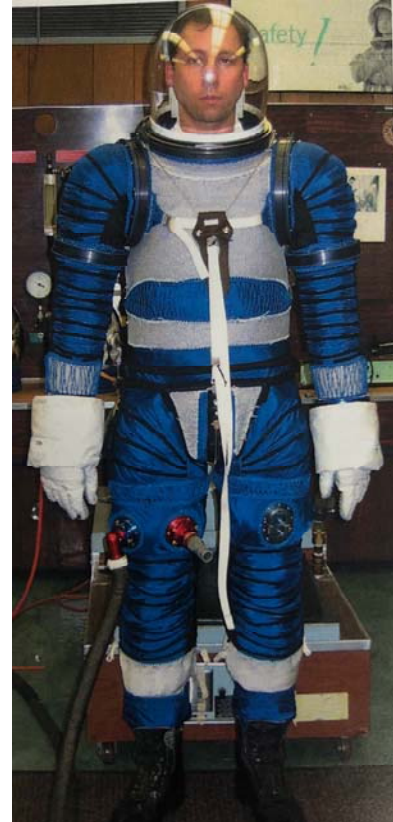
Figure 2. The CSSS derived EM-ACES suit included shoulder bearings. 6
