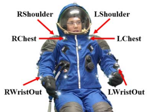
Figure 5. motion capture marker layout of a suited pressurized subject.
