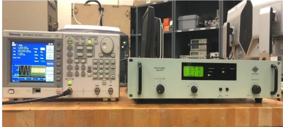
Figure 3.3 Tektronix function generator (AFG 3051C) and Brüel and Kjær power amplifier (Type 2718)
