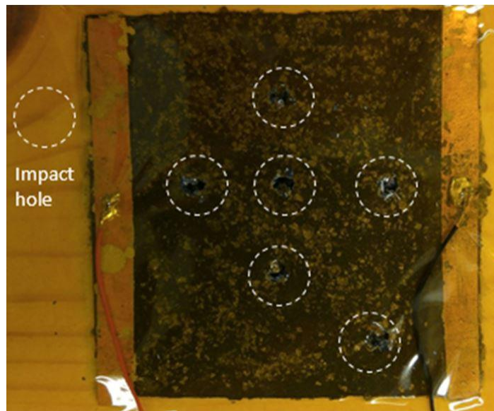
Figure 6.12 2.5\text{ in} \times 2.5\text{ in} coarse graphene sensor with Kapton tape, after addition of six 3 mm holes.
