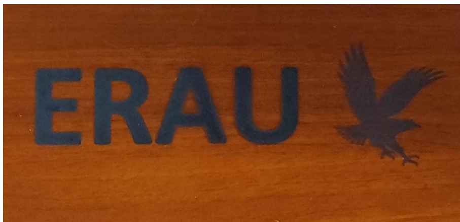
Figure 2.1 Inkjet printing of Embry-Riddle Aeronautical University logo with CNT ink.
