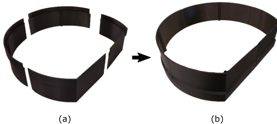
Figure 4. The printed payload housing core. (a) Four sections before bonding and (b) after bonding.
