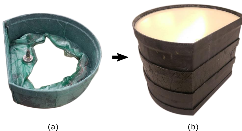
Figure 5. (a) Vacuum bagged carbon fiber prepreg on the printed core. (b) Carbon fiber reinforced composite payload housing assembly.
