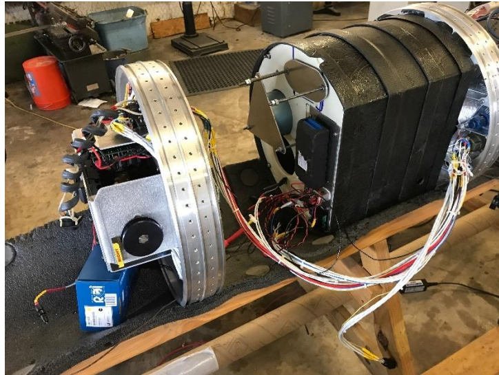
Figure 7. The payload housing assembly installed in EXOS SARGE rocket Adapted from “ SARGE Update: 7/31/17. EXOS Aerospace” by L. Gregory, 2017, EXOS Aerospace .
