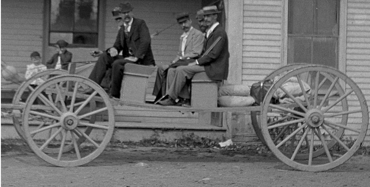
The wagon used to take people into the wilderness were built somewhat different. They generally had two rows of seats and no springs. The body was flexible so the ride was a bit more comfortable but still allowing the wagon to be picked up over boulders or easily pulled out of the mud. Courtesy of Lucius Merrill Collection Bangor Public Library Dated September 31, 1894
