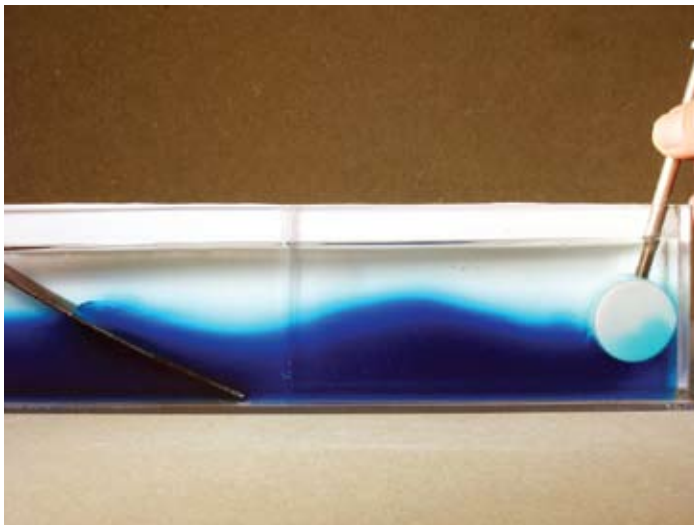
Figure 5.2. Internal waves. An internal wave at the interface between two fluids of different densities (dense blue water and less-dense clear water). A wave paddle that can be used to demonstrate resonance (see text) is shown on the right side of the tank, and a piece of plastic that simulates shallowing topography is shown on the left side of the tank.
