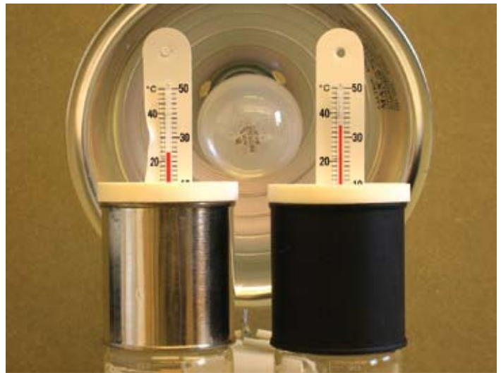
Figure 4.1. Setup for Activity 4.1. The thermometers show the difference in temperature between the black and shiny cans after the cans have been exposed to a light source.
