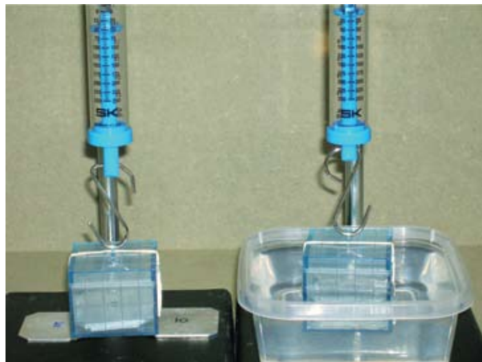
Figure 3.1. Apparatus for Activity 3.1 in air (left, with two weights lying on the table) and in water (right).
