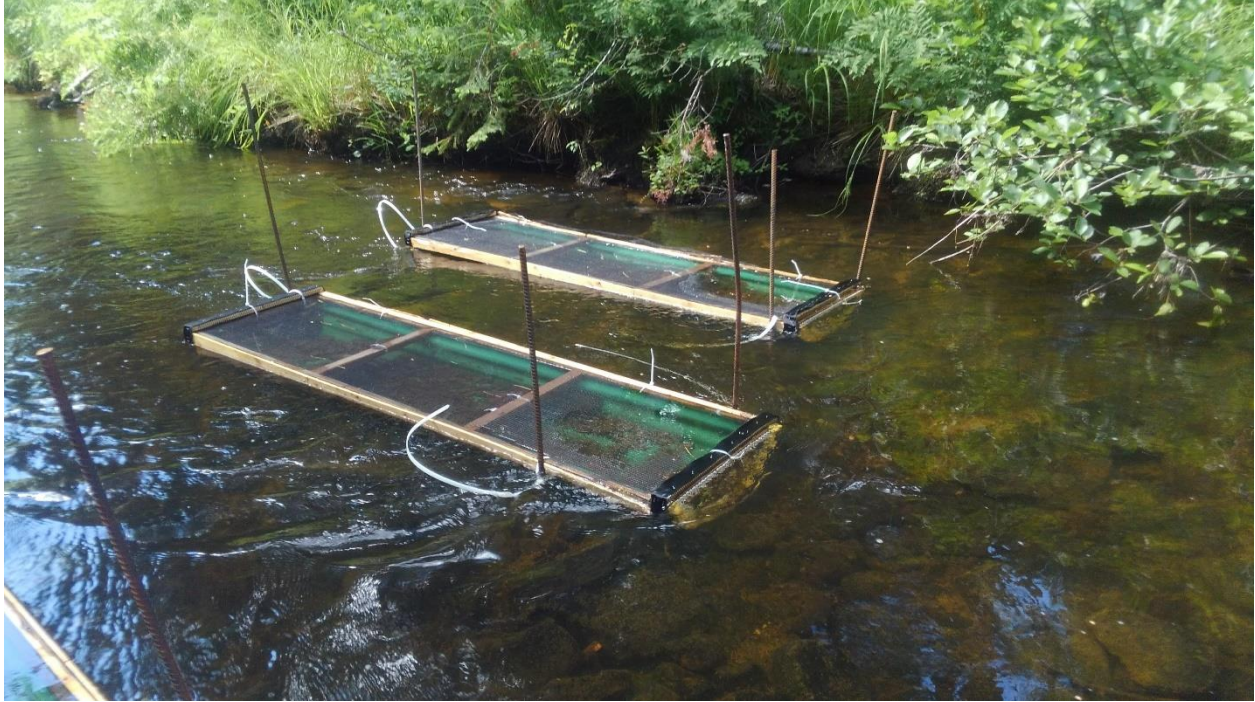
Figure 4.1 Image of stream channels placed in Sunkhaze Stream, Maine, during the Summer 2018 field season. Stream channels were placed directly in streams to mimic natural stream conditions. Mesh attached at both ends allowed for stream water to flow through the channel, supporting natural invertebrate colonization and a mesh lid allowed access to the channels.
