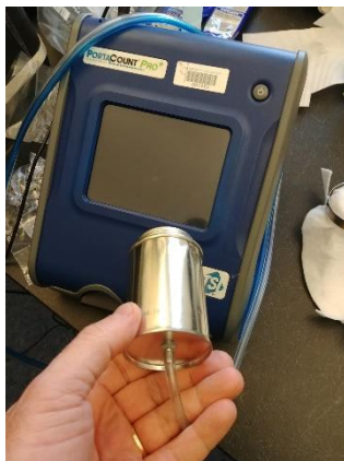
Figure 2: Chamber Base hose port sealed with an o-ring
