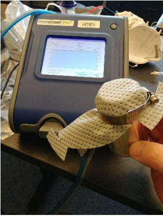
Figure 3: Test material sealed to chamber
