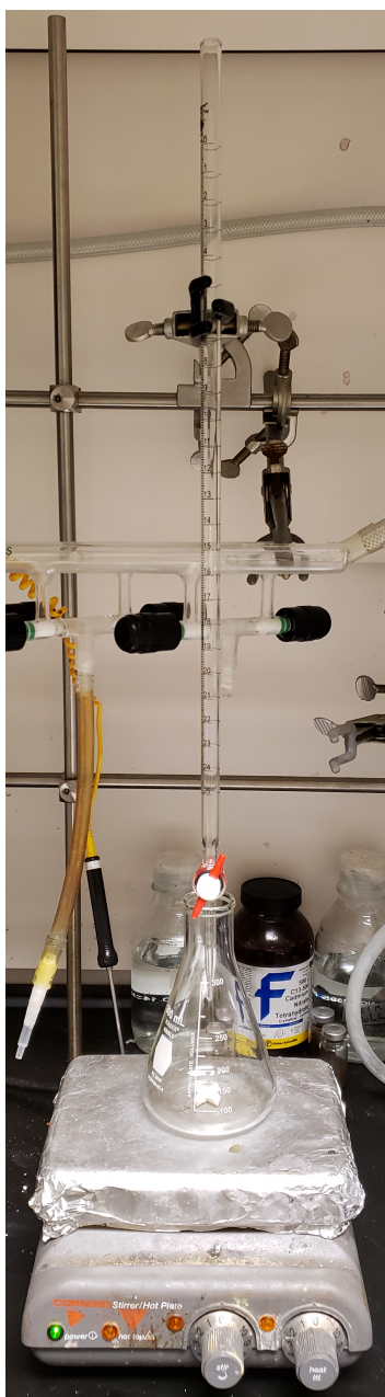
Figure 2.2: Typical reaction set up for ZnO NCs using acid base hydrolysis using a glass Burette that allows the solution to be add drop-wise into an Erlenmeyer flask with constant magnetic stirring. The entirety of the reaction is performed in air at room temperature
