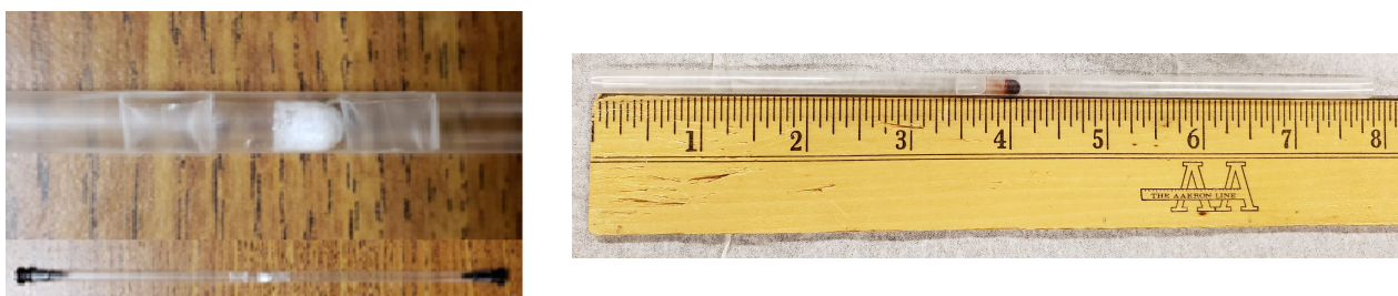
Figure 2.9: (left) How a proper sample should look when packed correctly and loaded into the sample holder. (right) Samples should be seated 4" from the top of the sample holder for easy centering in the MPMS.
