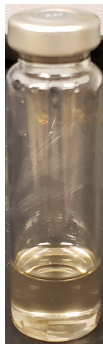
Figure 2.1: Typical experimental setup using a round bottom flask and water cooled condenser (left). The round bottom flask is heating using a hemispherical heating pad while utilizing magnetic stirring and temperature readings are measured using a thermal couple. All N_2 gas is delivered through a Schlenk line. A typical crimp vial with Se powder and TOP under N_2 atmosphere (right). The solution will become yellowish in color as the Se dissolves into solution
